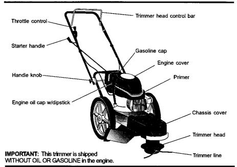
Trimmer head control bar - must be held down to the handle to engage trimmer head. Release to stop the trimmer head. Primer - pumps additional fuel from the carburetor to the cylinder for use when starting a cold engine.
